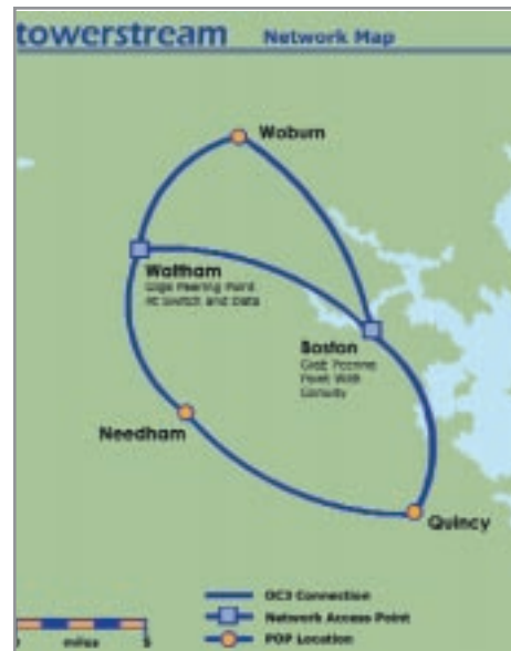
TowerStream's fault-tolerant wireless backbone features redundant links and dual peering points for maximum network availability.
