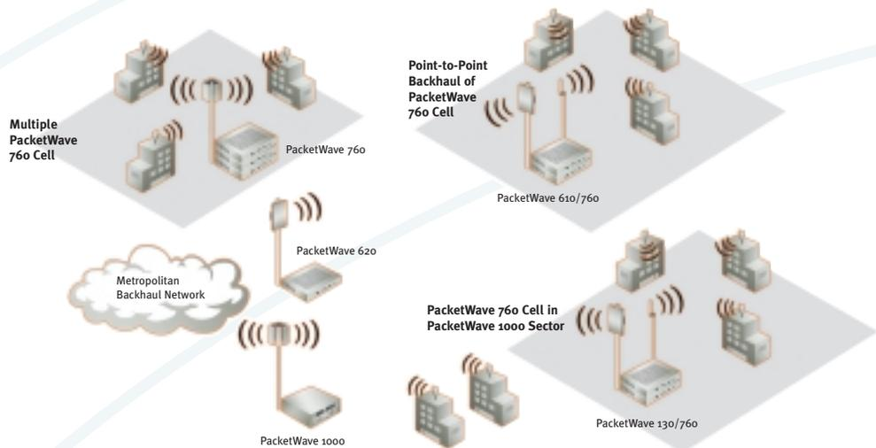
Aperto's Packetwave 760 operates as a multi or single sector base station or as a component of Aperto's integrated family of products.
